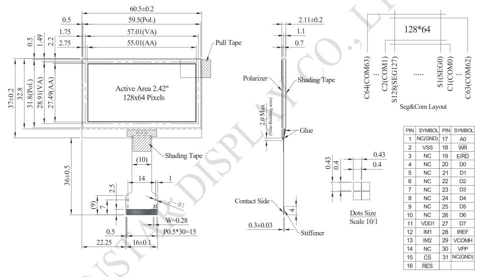
The non-specified tolerance of dimension is  $\pm 0.3$ mm.
